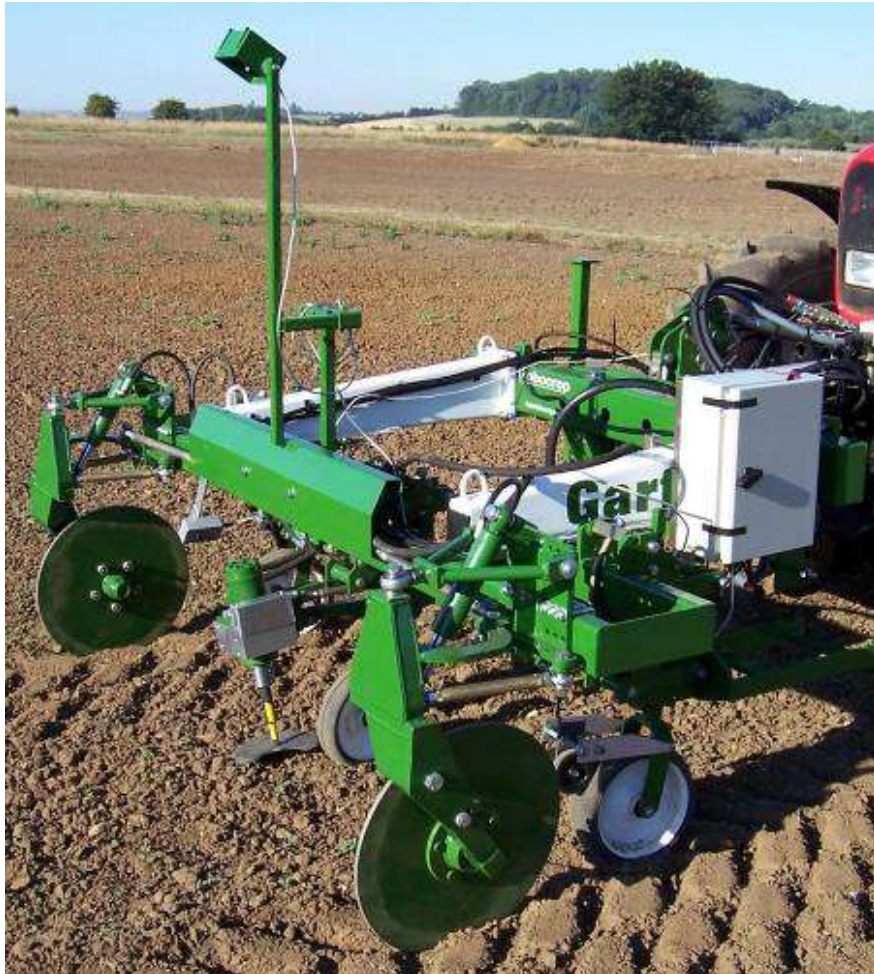
Figure 14 A 2m wide experimental toolframe designed and constructed by Garford Farm Machinery that was used for field trials and demonstration work.
