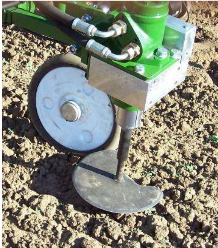
Figure 15 A hydraulically driven selective disc cultivation module fitted with a flat disc
