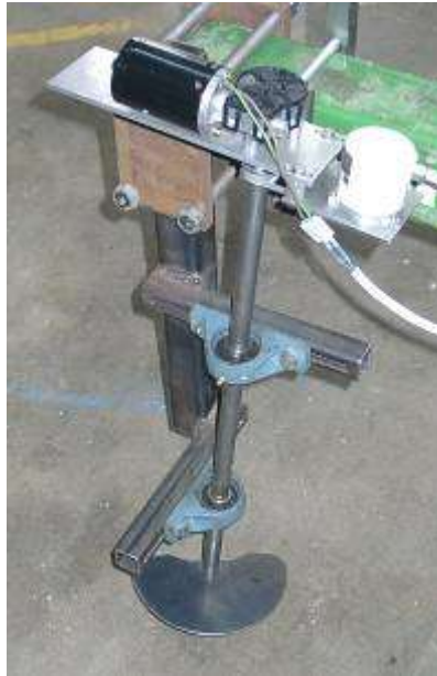
Figure 10: Electrically driven test rig for experimental development above ground
