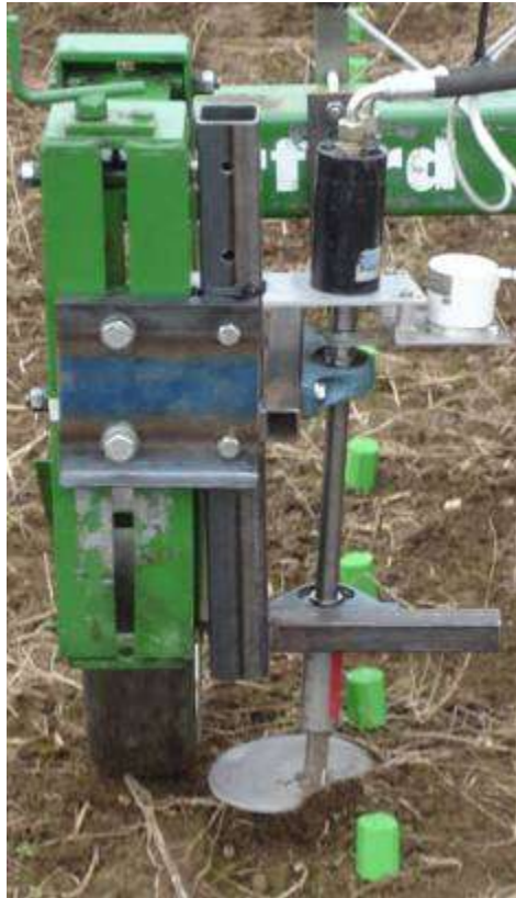
Figure 12 A single row field test rig with depth control and hydraulic drive shown operating on artificial plants above the soil surface.
