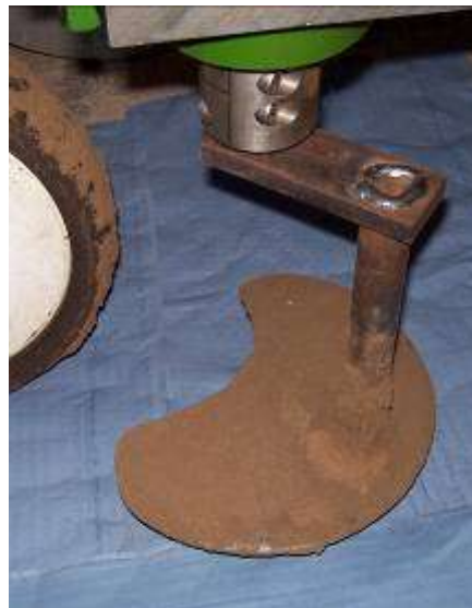
Figure 18 Cranked disc shaft modification to increase plant to shaft clearance
