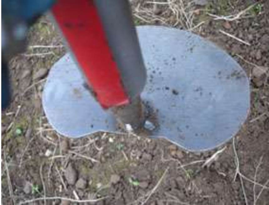
Figure 8 Rotating disc with cut out as used in early field trials
