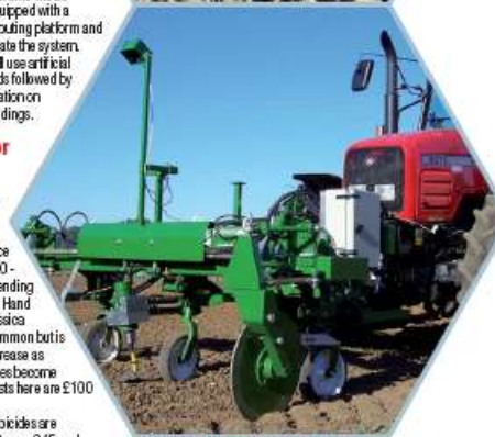
Top: the novel shallow cultivator has been successfully synchronized with a computer programme for the tracking of individual crop plants. Above: An experimental prototype in the field
